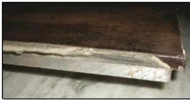
Fig. 2 Carbon Steel/Epoxy/Aluminium Laminated Metal Composite (LMC)
