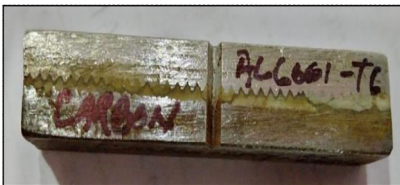
Fig. 10 Charpy Test Specimen of SAE 1042 Carbon Steel + Epoxy + Aluminium 6061-T6
