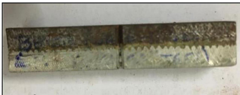
Fig. 9 Charpy Test Specimen of Carbon Steel + Epoxy + Aluminium 5083-H112
