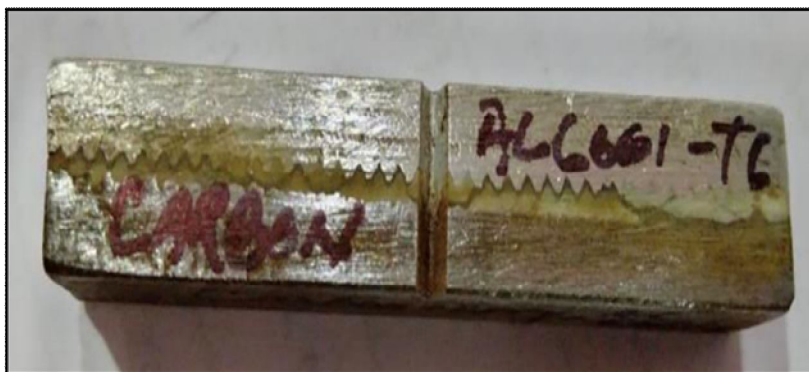
Fig. 10 Charpy Test Specimen of SAE 1042 Carbon Steel + Epoxy + Aluminium 6061-T6
