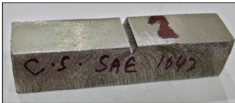
Fig. 7 SAE 1042 Carbon Steel Charpy Test Specimen
