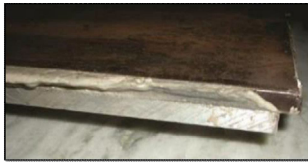
Fig. 2 Carbon Steel/Epoxy/Aluminium Laminated Metal Composite (LMC)
