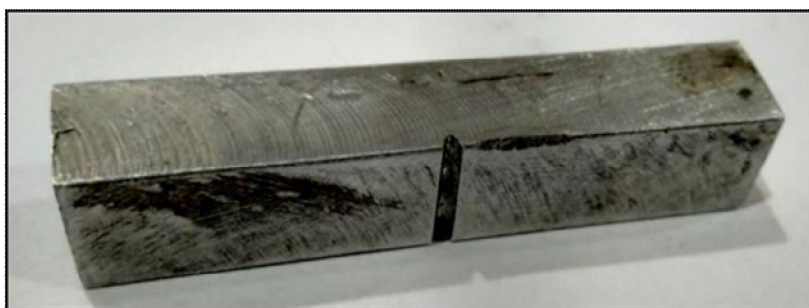
Fig. 8 Aluminium 6061-T6 Charpy Test Specimen
