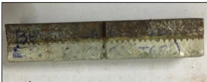
Fig. 9 Charpy Test Specimen of Carbon Steel + Epoxy + Aluminium 5083-H112
