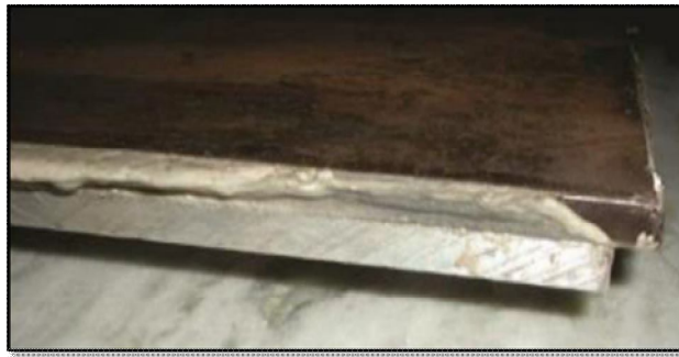
Fig. 2 Carbon Steel/Epoxy/Aluminium Laminated Metal Composite (LMC)
