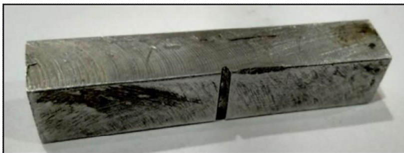
Fig. 8 Aluminium 6061-T6 Charpy Test Specimen
