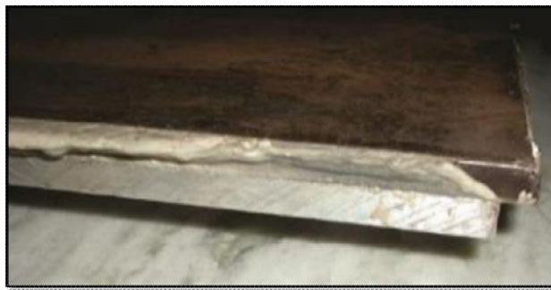
Fig. 2 Carbon Steel/Epoxy/Aluminium Laminated Metal Composite (LMC)
