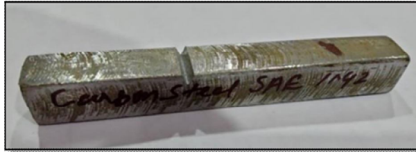
Fig. 3 SAE 1042 Carbon Steel Izod Test Specimen
