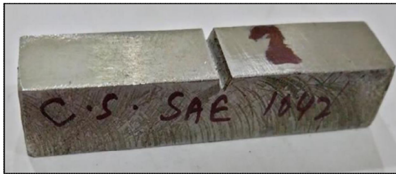
Fig. 7 SAE 1042 Carbon Steel Charpy Test Specimen
