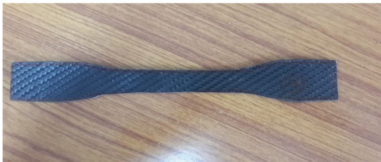
Fig. 7. Specimen wrapping with carbon fibre
