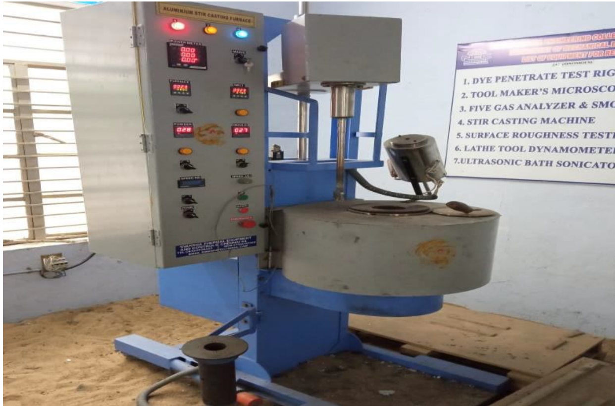
figure 1. stir casting equipment
