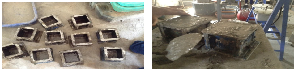
Fig –3.3 casting of cubes.
