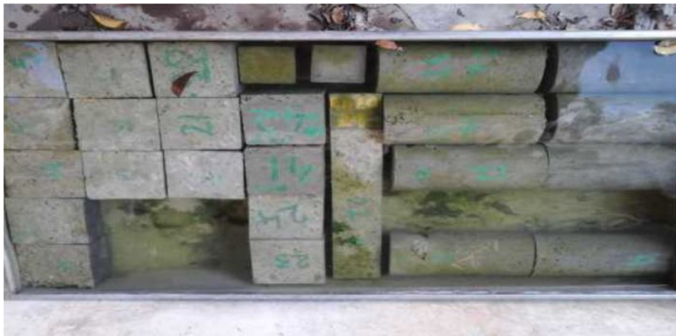
Fig – 3.6 curing of specimens.
