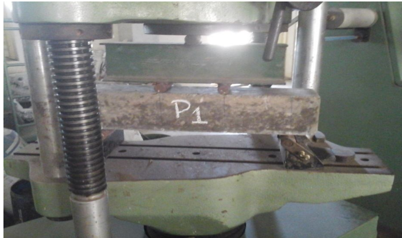
Fig 4.4 testing of specimens for split tensile strength
