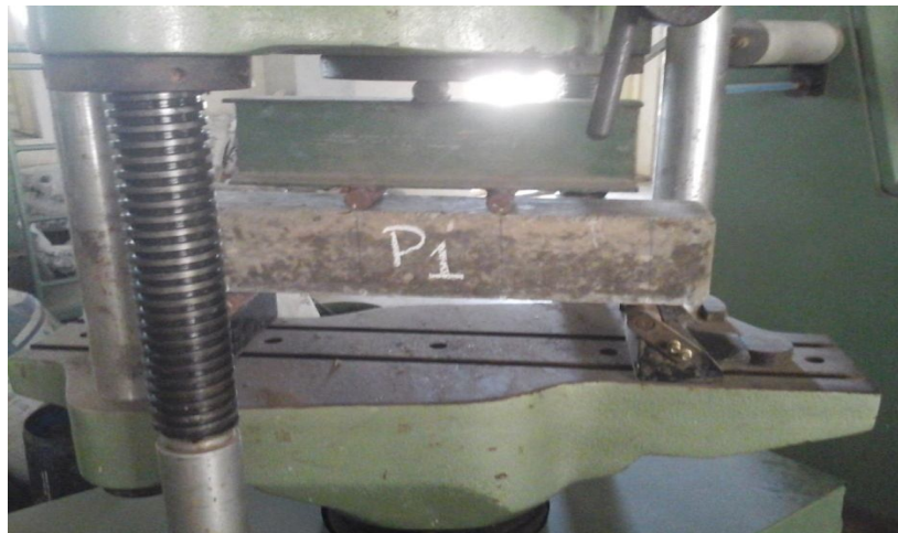
Fig 4.4 testing of specimens for split tensile strength
