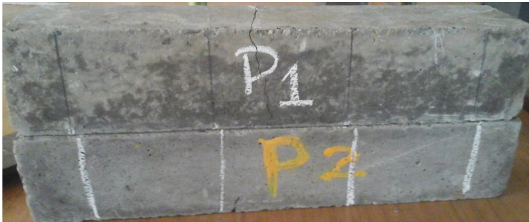
Fig – 3.5 casting of prisms and testing of specimens
