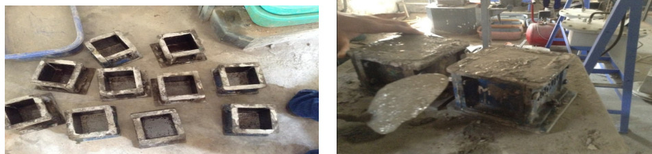
Fig –3.3 casting of cubes.
