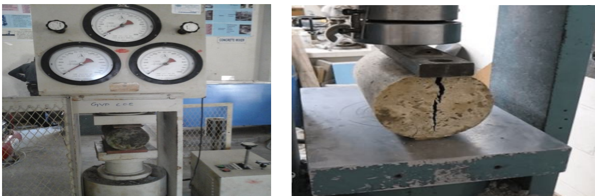
Fig 4.3 testing of specimens for split tensile strength
