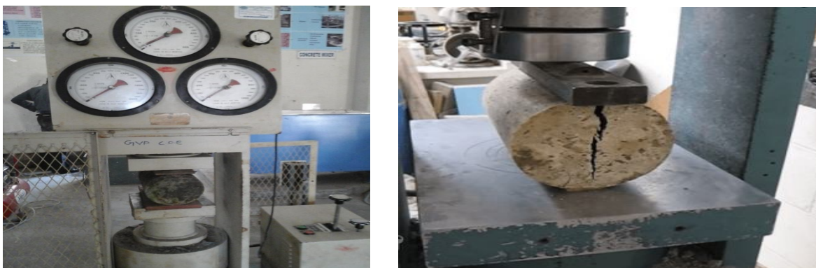
Fig 4.3 testing of specimens for split tensile strength
