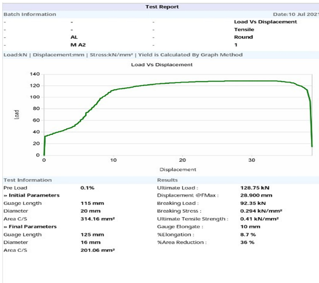
Graph 6: Tensile test graph For AI7075 + 4.5% of Nickel coated hBN
