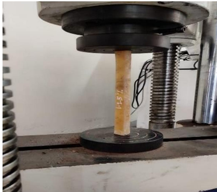
Fig. 5.3 Flat Sample Placed in the UTM for Compressive Test
