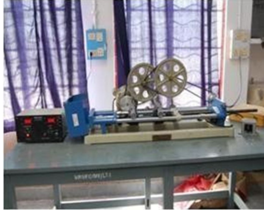
Fig 5.2 Tensometer used for testing tensile and bending strength
