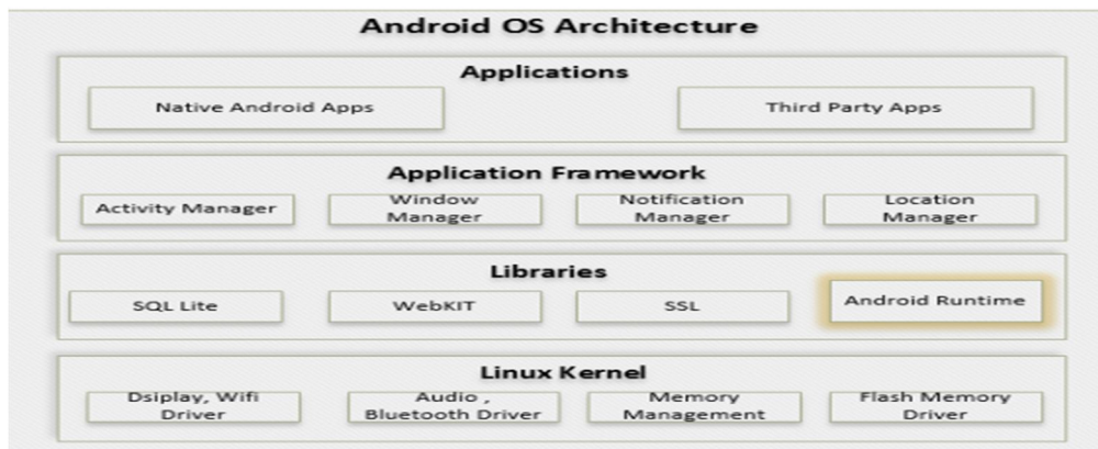
Fig.1. Android OS Architecture
