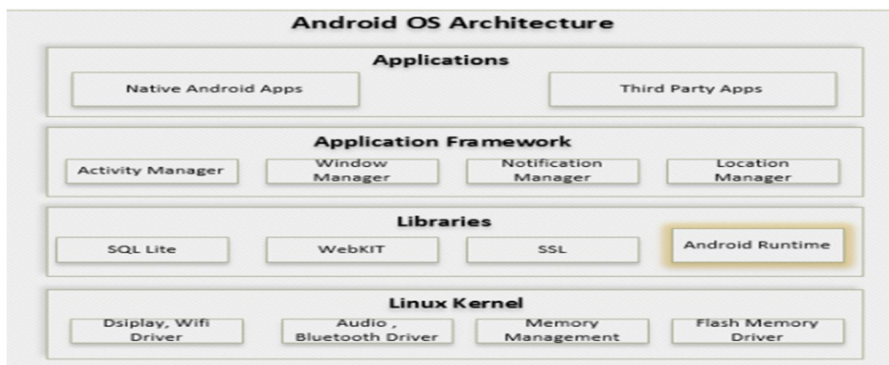
Fig.1. Android OS Architecture
