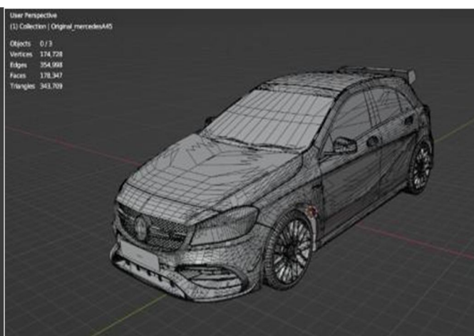
Fig. 11 Angle limit – 1 degree (178,347 faces)
