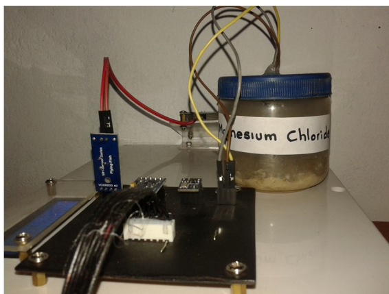
Fig. 10 Calibration Process of the Humidity Sensor with Magnesium Chloride
