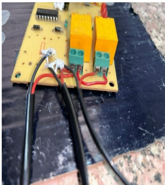
Fig.6. Arduino uno with relay module
