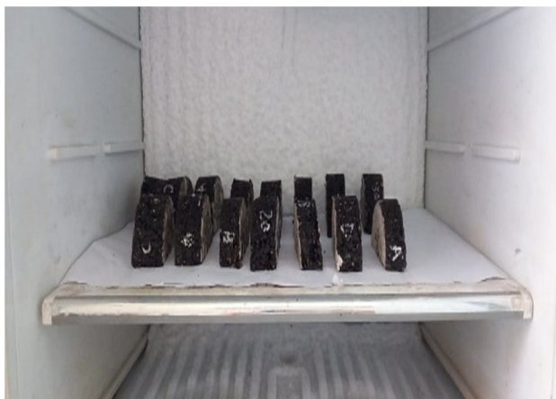
Figure 5: Brittle condition -18^{\circ}\text{C}
