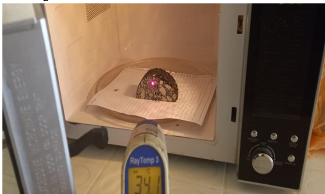
Figure 4: Surface temperature monitoring using infrared thermometer
