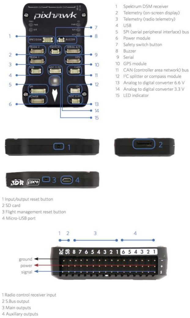
Fig: 6.10 Flight Controller Detailed Picture
