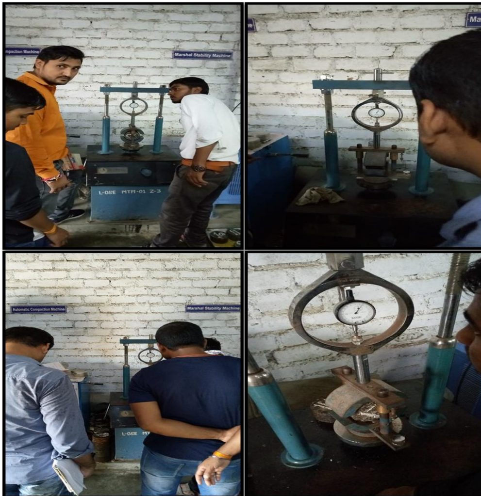
Figure:- ITS Testing in dry condition
