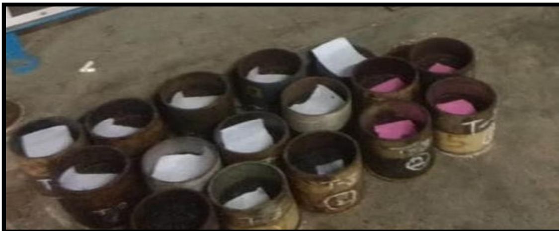
Figure:- Curing of specimen in the mould for 24 hours at room temperature
