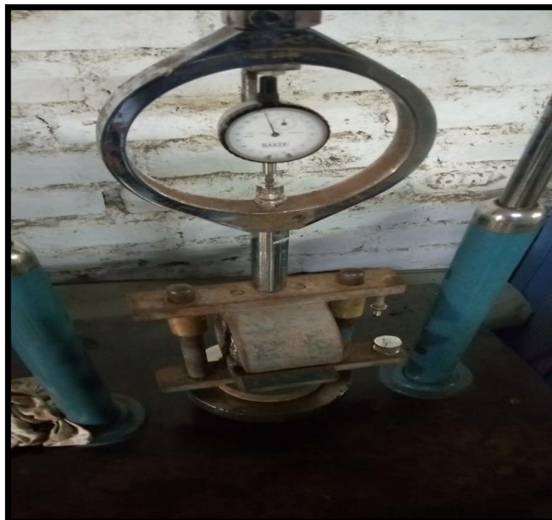
Figure-: Calibrated proving ring & dial gauge
