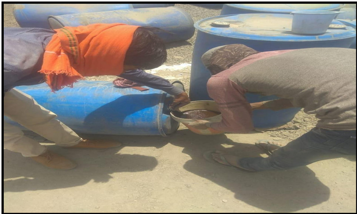
Fig:- Sampling of Bitumen emulsion from stock yard
