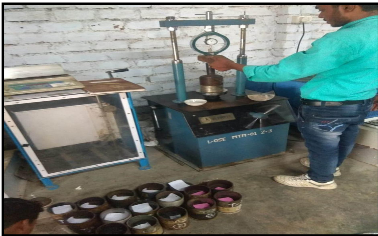
Figure:- Extrusion of specimen from the mould by using marshall machine
