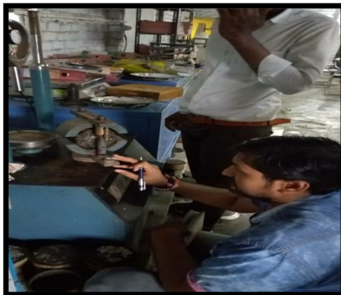
Figure-: Mould placing in the machine for ITS testing
