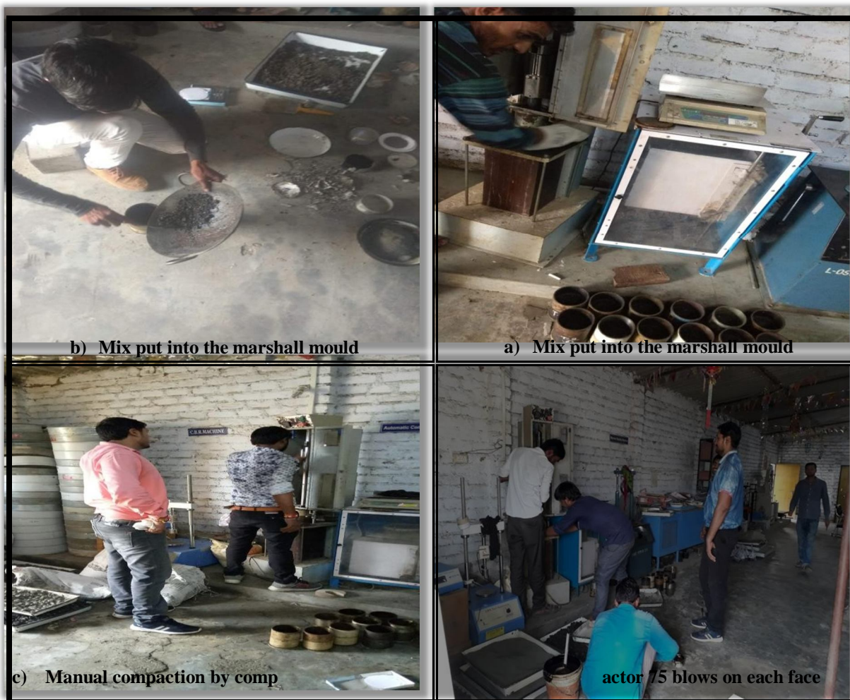
Figure:- a) Mix put into the marshall mould b) Mould place in the compactor machine c) Manual compaction by compactor 75 blows on each face
