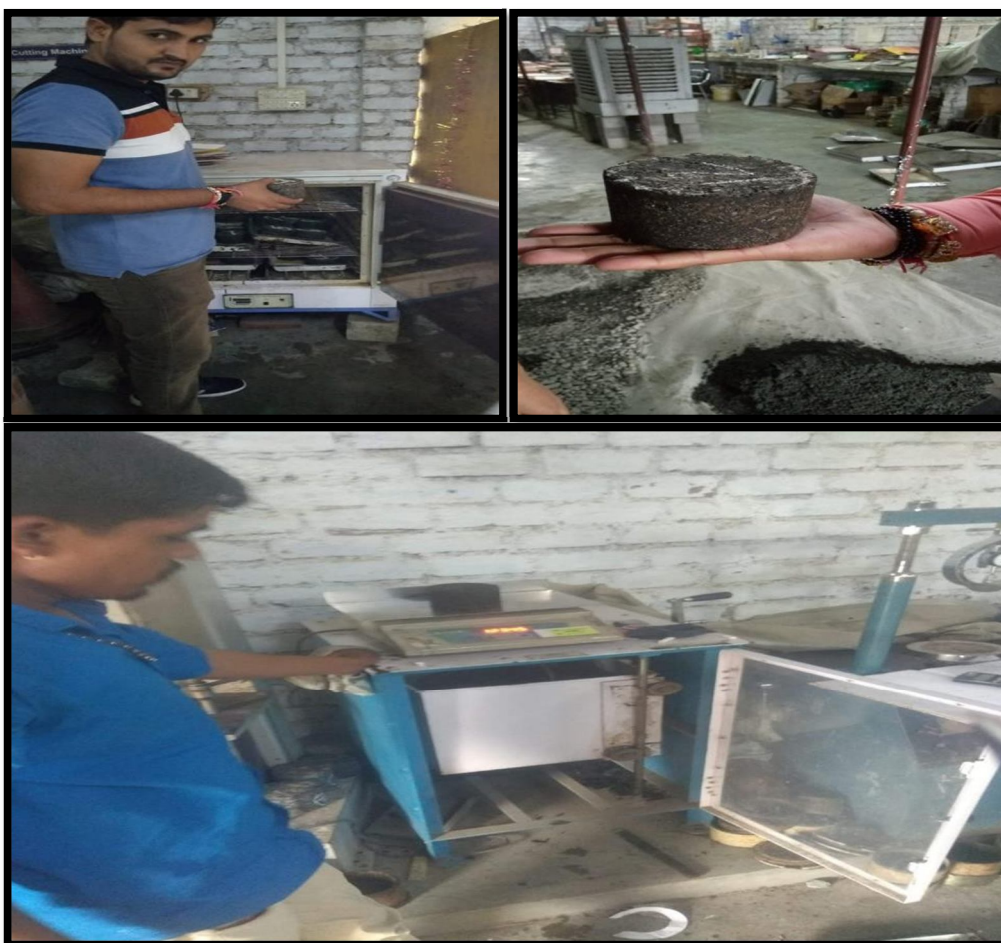
Figure-: Casted Mould put in hot air oven maintained at 40°C for 72 hours
