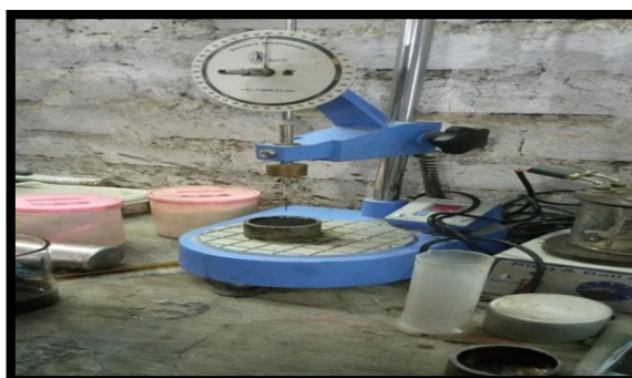
Figure-: Penetration test in site laboratory
