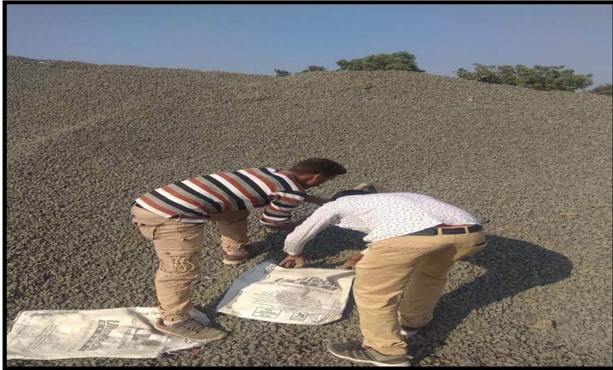
Figure-: Sampling of 20 mm aggregate at Sunera Camp
