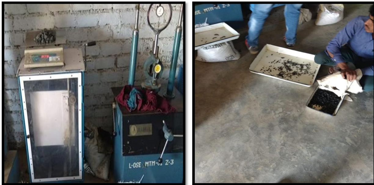
Figure-: Specific gravity and water absorption test on 20 mm down aggregate
