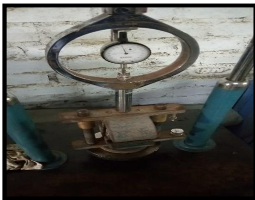
Figure-: Take the dial gauge and proving ring initial reading
