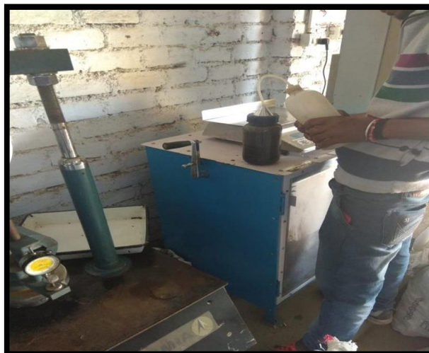
Water absorption and specific gravity test at site laboratory
