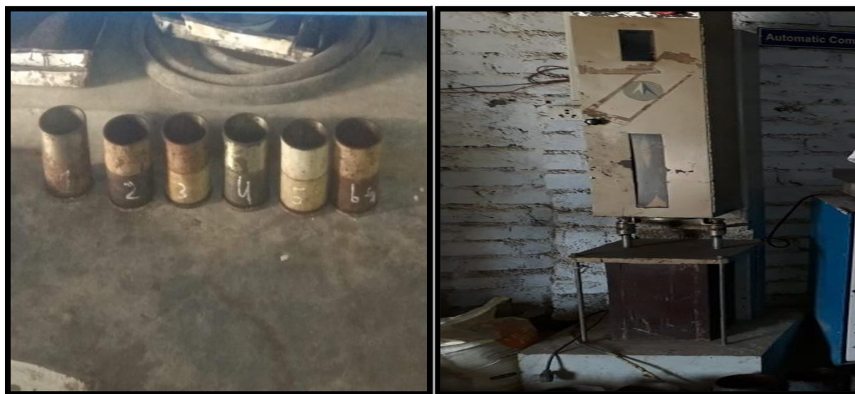
Figure:- 100 dia marshall mould & Compactor
