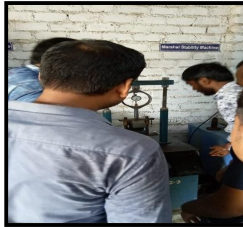
Figure:- Machine operated at the speed of 55 mm/min
