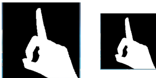
Figure 4 (a) Image after binarise. (b) Image after segmentation and resizing.
