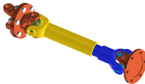
Fig. 1 Universal joint and drive shaft assembly
