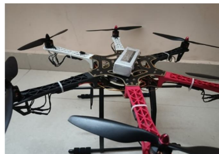
Figure. Assembled Drone
