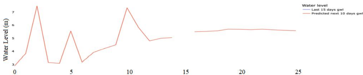
Figure 9b: Plotting last 15 days and next predicted 10 days of Rajshahi by LSTM
