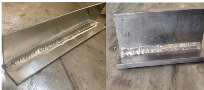
Fig 9 welding process completed in t-joint and corner joint method.
