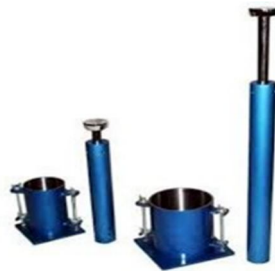
Figure 5: Standard Proctor Compaction Test Apparatus.
