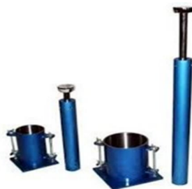
Figure 5: Standard Proctor Compaction Test Apparatus.
