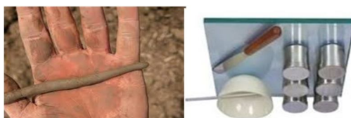
Figure 2: Plastic Limit Sample and Test Apparatus
