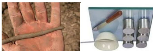
Figure 2: Plastic Limit Sample and Test Apparatus
