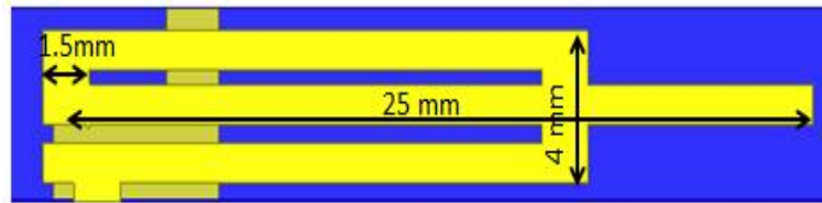
Fig (3): Modified Bending Dipole with measurement
