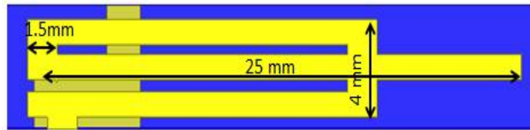
Fig (3): Modified Bending Dipole with measurement
