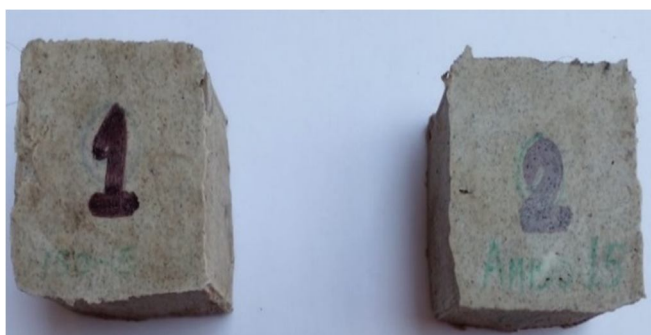
Figure 2: Isotropic/Unstructured (MRE-1) and Anisotropic/Prestructured (MRE-2)
