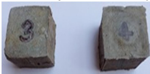
Figure 3: Isotropic/Unstructured (MRE-3) and Anisotropic/Prestructured (MRE-4)
