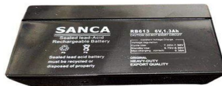
Fig.6 Lead Acid Battery
