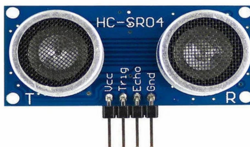
Ultrasonic Sensor – HC-SR04
