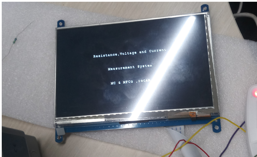
Fig.11 LCD Display on Measurement mode
