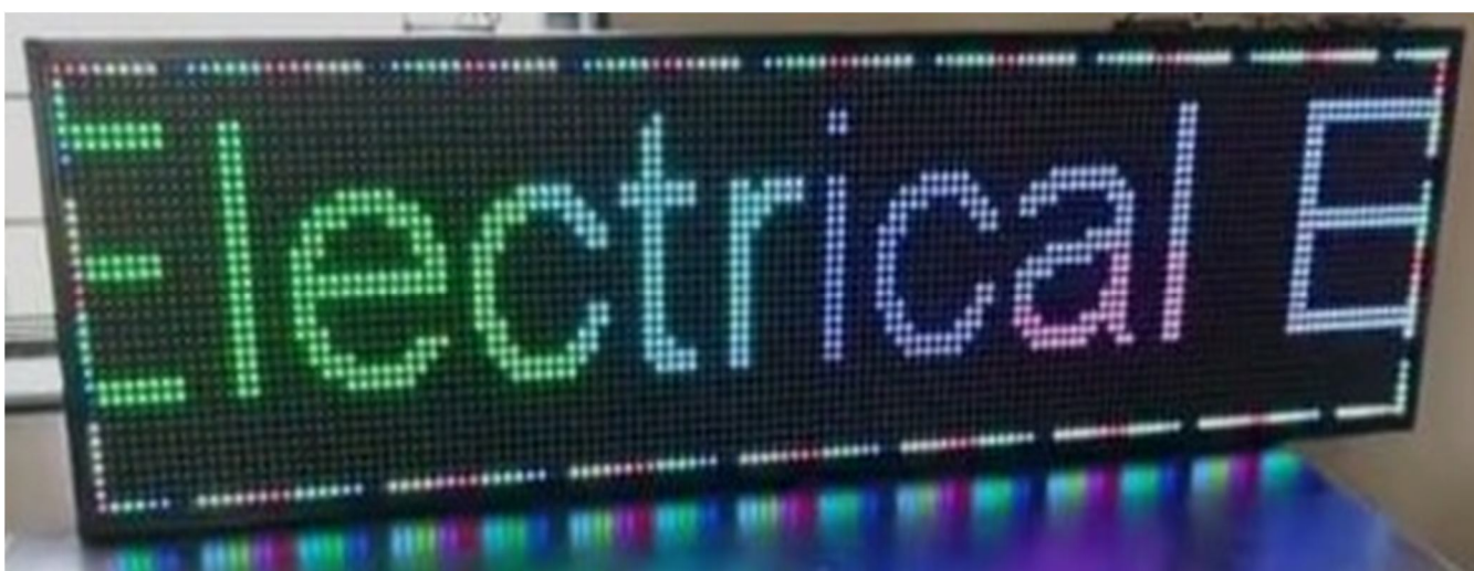
Fig. 2 P10 LED Display
