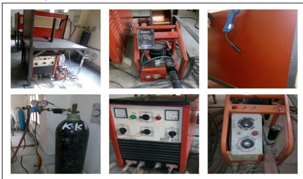
Figure 4: Different part of MIG welding setup
