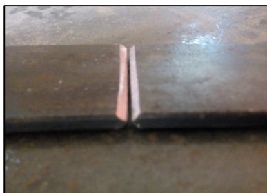
Figure 4: Prepared double V- groove shape joint for butt welding
