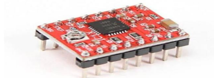
Fig-7: A4988 Motor Driver
