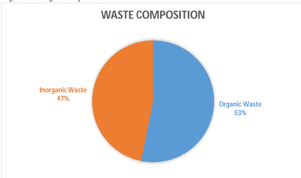
Figure 4.0: A Pie-chart Representing the Organic and Inorganic Components of Yenagoa Municipal Waste
