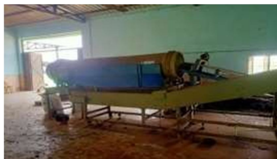
Fig- 1.4 Waste separator
