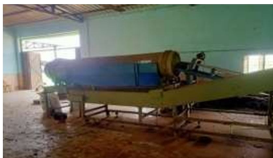
Fig- 1.4 Waste separator
