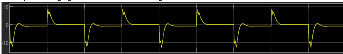
Fig 7 Ringing effect during switching
