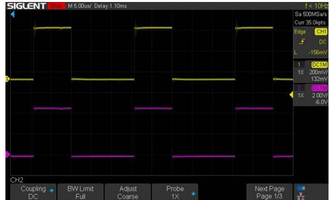
Fig.12. Gate signals of S1 and S2
