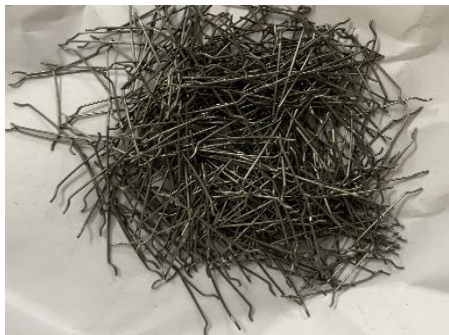
Fig.4.Hooked End Steel Fiber
