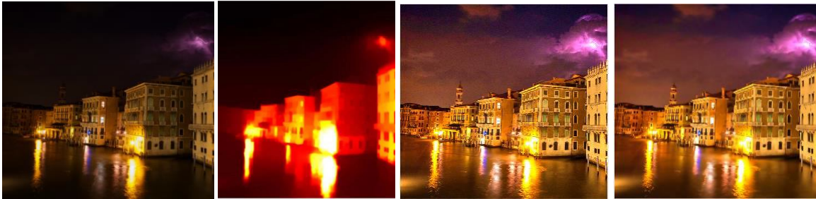
Example of visual performance (Figure 5). One, the original picture; two, the DCP map; three, the darkened image; and four, the denoised image.
