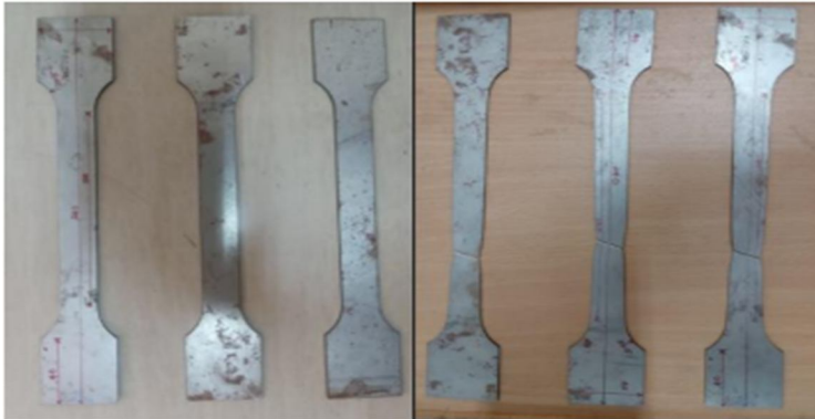
Figure 2 Coupon Test Specimen
