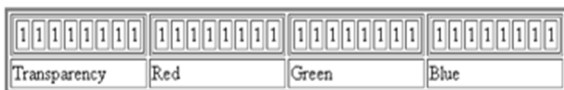
Fig: BIT Transferred for Red, Green and Blue plane (24bit=8bit red;8-bit green;8bit blue)
