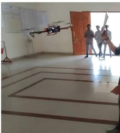
Fig. 4 shows the obstacle avoidance system being tested
