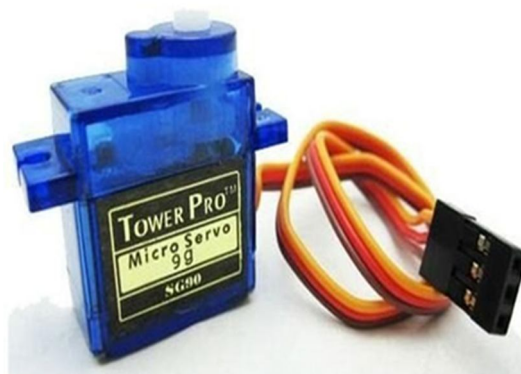
Fig. 4 Servo Motor (Tower Pro SG90)
