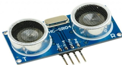
Fig. 2 Ultrasonic Sensor (HC-SR04)
