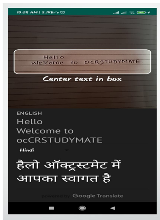
Fig 7.2.1: Image capturing & translating text for handwritten text
