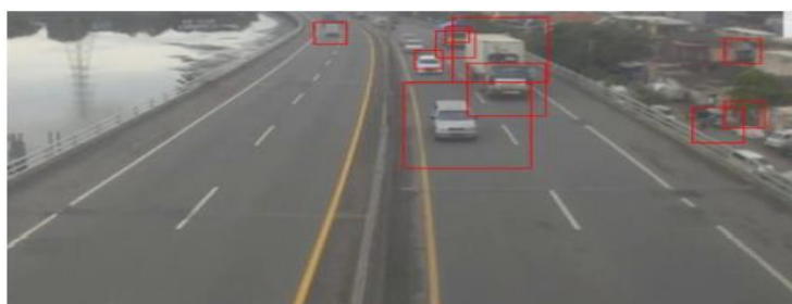
Fig4: Image showing bounding boxes of detected cars in the lane
