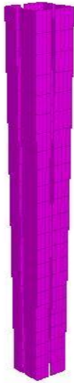
Fig. 6: Single Core Shear wall with 12.5 % opening and I = 1.5 (highest importance factor)
