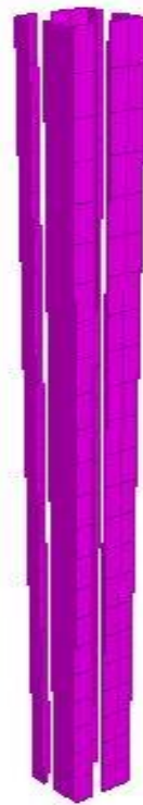
Fig. 8: Single Core Shear wall with 25 % opening and I = 1.5 (highest importance factor)
