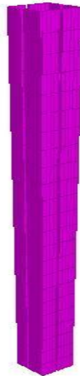
Fig. 5: Single Core Shear wall with 10 % opening and I = 1.5 (highest importance factor)
