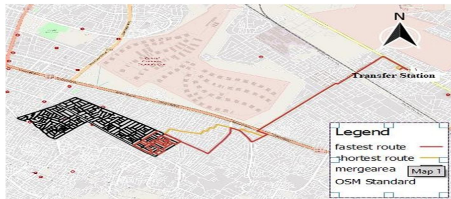
Fig-7: Optimized solid waste collection vehicle route
