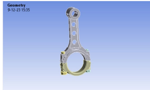
Figure 16: Geometry of optimized structure connecting rod
