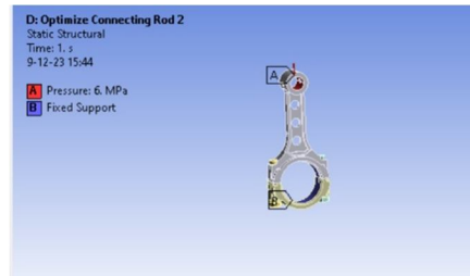
Figure 18: Boundary condition of the optimized structure of connecting rod
