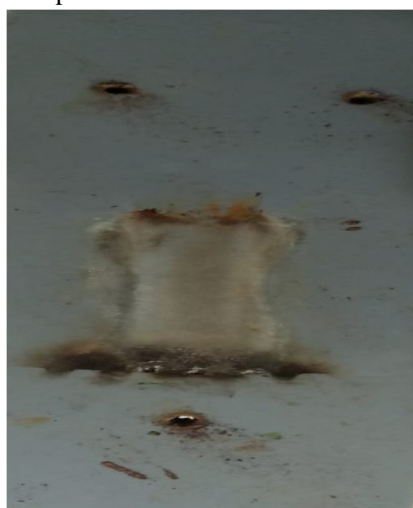
Fig 5.1 sample after 100 hours IPTE test
