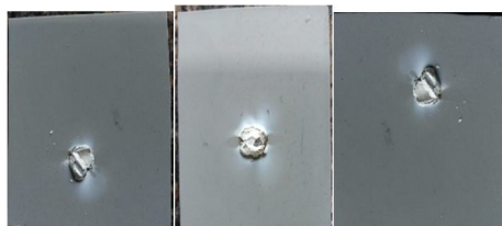
Fig 4.12: samples after the dry arc resistance test
