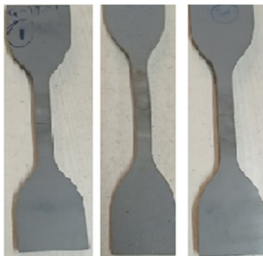
Fig 3.10: dumbbell shaped samples.
