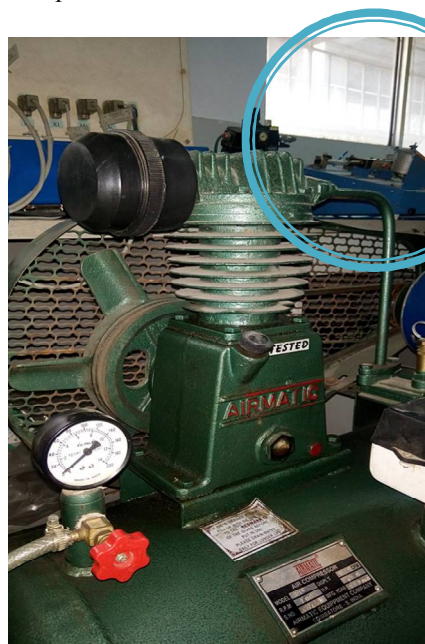
Figure 3.1: Design of actual fins body on the compressor head.
