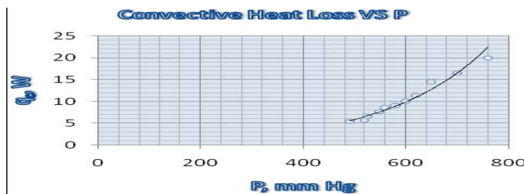
Figure 2.8: Effects of reduction in pressure on convective heat loss by solid cylindrical fin [3]
