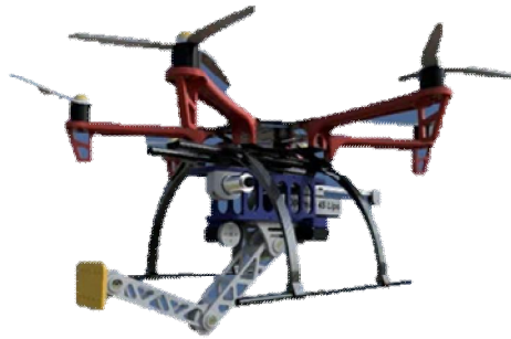
Fig.1 Design of UAV equipped with the manipulator [6]
