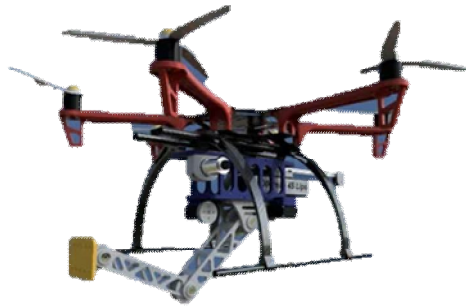
Fig.1 Design of UAV equipped with the manipulator [6]
