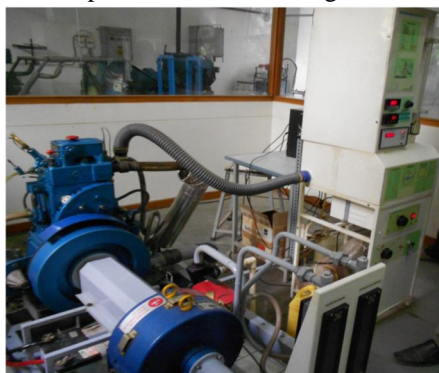
Fig. 1 Single cylinder diesel engine test rig
