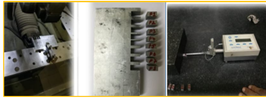
Figure 3.1: M/c Setup, work-piece and Ra measurement system
