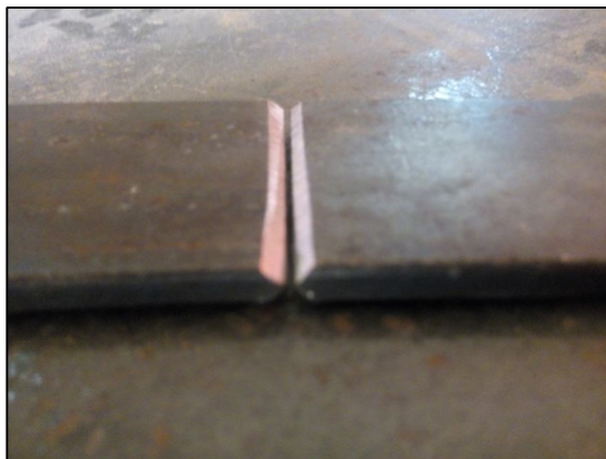
Figure 2: Prepared double V-groove shape joint for butt welding
