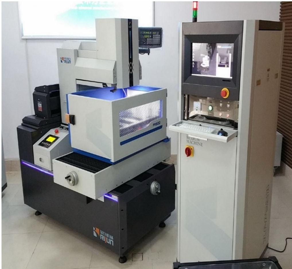
Fig.2. Wire EDM Machine
